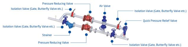
Pressure Reducing Valves reduce pressure to setted downstream pressure value without affecting upstream pressure value at pressure chambers and supplying lines.
