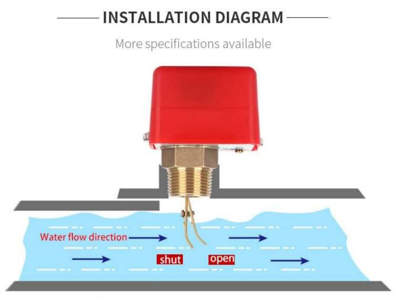
Single-pole double-head micro-movement working state, when the flow rate rises to the switching value, terminal 1-2 is connected; when the flow rate drops to the lower switching value, 1-3 is connected
