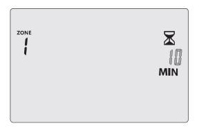
Press the + or — button to set the desired watering duration time.
