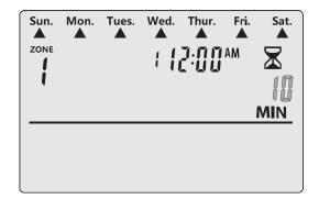
Press the + or - button to adjust the watering duration time, then press the ▶ button to move forward to the next option.
