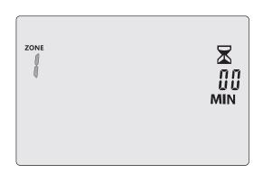
Press the + or - button to select a zone, then press the button to move forward to the next option.
