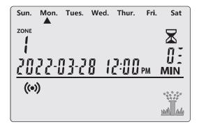
**Display in Irrigation Process:** The screen displays the current time and date, the serial number of the zone, and the remaining watering time. You will see the icon of the sprayer flashing.
