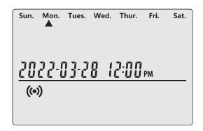
**Display in Auto Mode:** The screen displays the current time and date.
