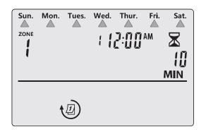
Press the → or — button to select days of the week. You will see the display characters flashing. Press the ▶ button to move forward to the further setting.
