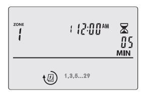
Press the + or - button to select the odd numbers of 1,3,5...29. You will see the display characters flashing. In that case, press the ▶| button to move forward to the next option.
