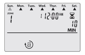
Press the → or — button to activate or forbidden irrigation on the designated day which is flashing, then move to the setting of the next day.
