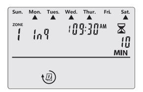
• In auto mode and simultaneously in the non-irrigation process, press the → or — button to enter the inquiry interface. You will see the characters "Inq" (inquiry) displaying and the information about the watering schedules of this zone.
