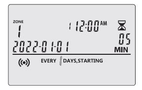
● Press the + or — button to set a number of days for the time interval. You will see the display character flashing. In that case, press the ▶| button to move forward to the next setting.
