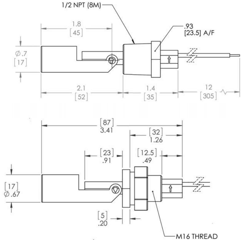
The **SML** series is a horizontal mount level switch ideal for monitoring Water and Oil levels
