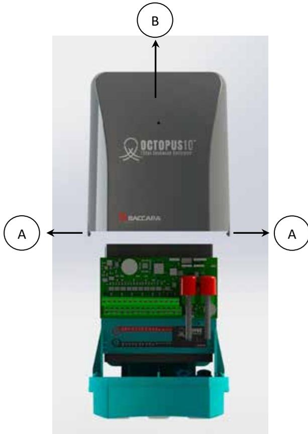
Once the controller is firmly mounted to its bracket, remove the controller's cover by slightly pushing out the two tabs in its side [A], and pulling up the cover [B].
